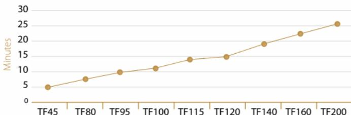
Predicted heat up times for cylinder based on test procedures defined in BS1566:2002 for type P cylinders.
